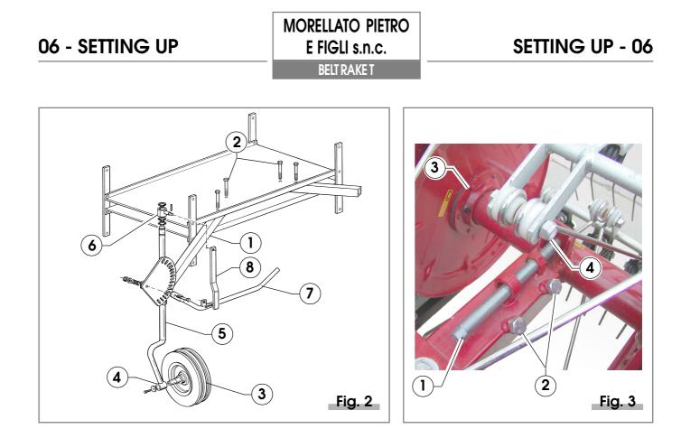
**3.** Turn the rocker arms to their operational position and fasten each of them with the preceding twin tie rod with the screw and locknut preassembled in the tie rod (figure 3, item 4).
