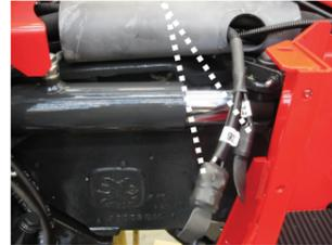
Lichtmaschine X13.1 X13.2 X13.3
